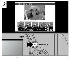
Place an "m" mark under all the images you do not want to record and then press the "MENU/OK" button to record the remaining images.
